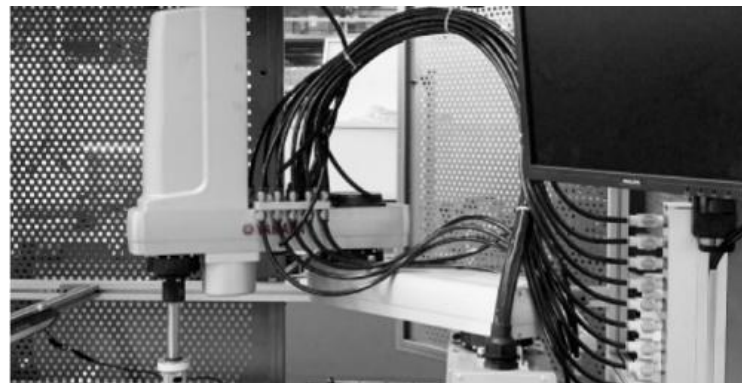
Camera robot positioning system
